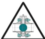
By tightening the stay-bolts when the disc is closed, the liner will be compressed in a wrong position. An excessive closing torque and leakage will result. Open completely the disc (Fig. 8). Ensure that the piping is aligned. Tighten diagonally opposite the nuts.
