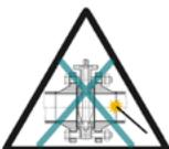
The valve should never be installed between flanges which are not parallel to each other.
