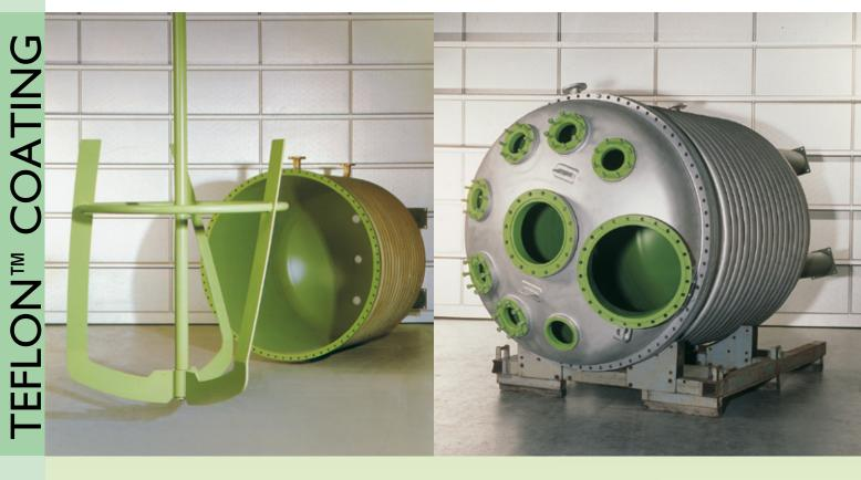
In the spraying sinter procedure (airless and compressed air process), Gutbrod works with Teflon $^{\text{IM}}$  Coating. The coating is sprayed on and then "sintered" at 220°C to 420°C.
